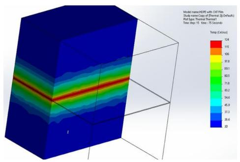
**Figure 1:** Results of transient heat transfer simulation in Solidworks. Maximum temperature of 124C at 75 seconds.
