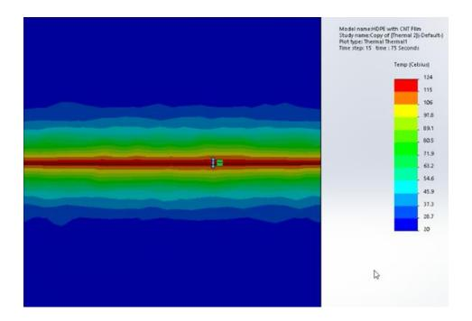
**Figure 2:** Line covers an approximate range for the melting of HDPE. The line length was ~1.2mm, and the thickness of the film was 0.25mm.
