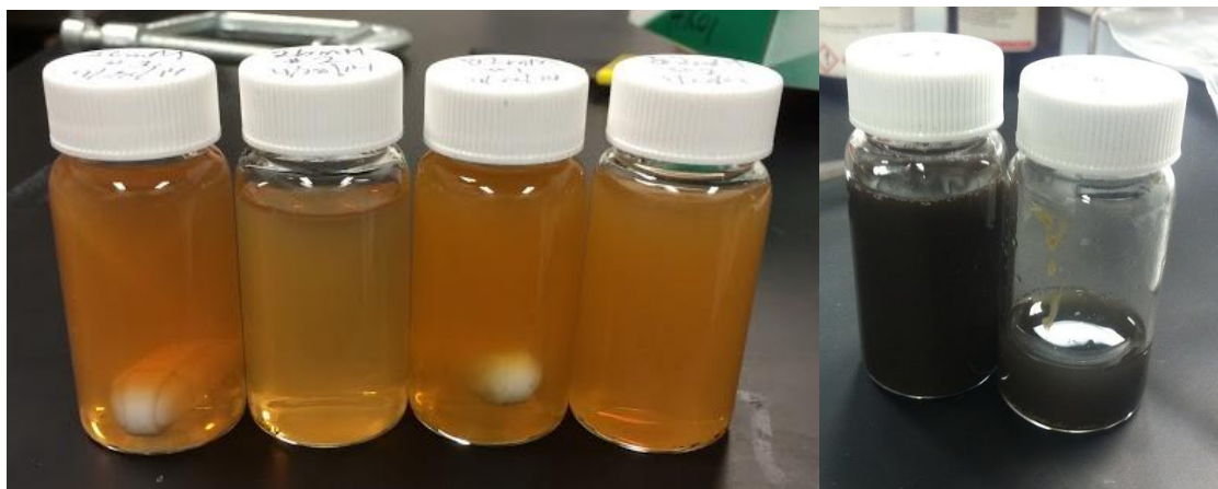
Figure 7: The orange vials are those with synthesized silver nanoparticles suspended in chitosan/acetic acid solution. The brown vials were likely damaged by UV exposure during a weekend by a window.
