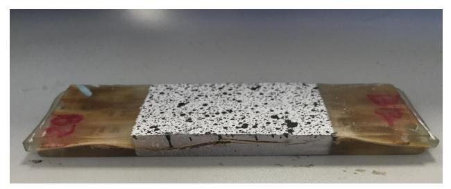
Figure 9: BFRP sample that fractured along its side due to poor fiber/epoxy adhesion
