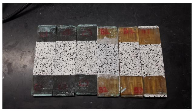
Figure 7: Samples with primer and black speckles prior to tensile test
