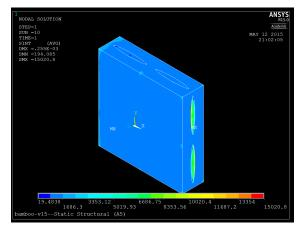
Figure 5: A snapshot of the stress intensity during a tensile test. This picture shows the final point of the tensile test
