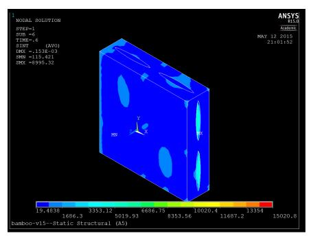
Figure 6: A snapshot of the stress intensity during a tensile test. This picture shows a point in time in the middle of the tensile test
