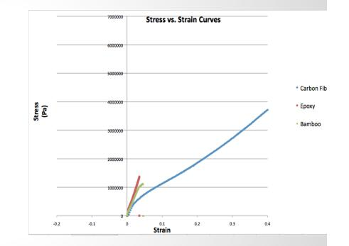
Figure 13: Tensile Test of Samples
