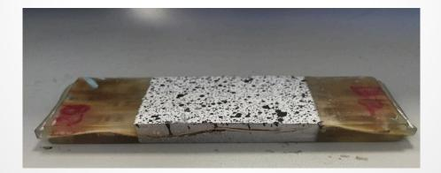
Figure 14: Example of Delamination
