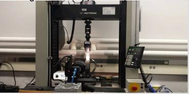
Figure 12: Composite in Tensile Test
